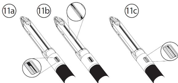
The knife can be retracted by pushing the “Reverse” button forward on the device.
